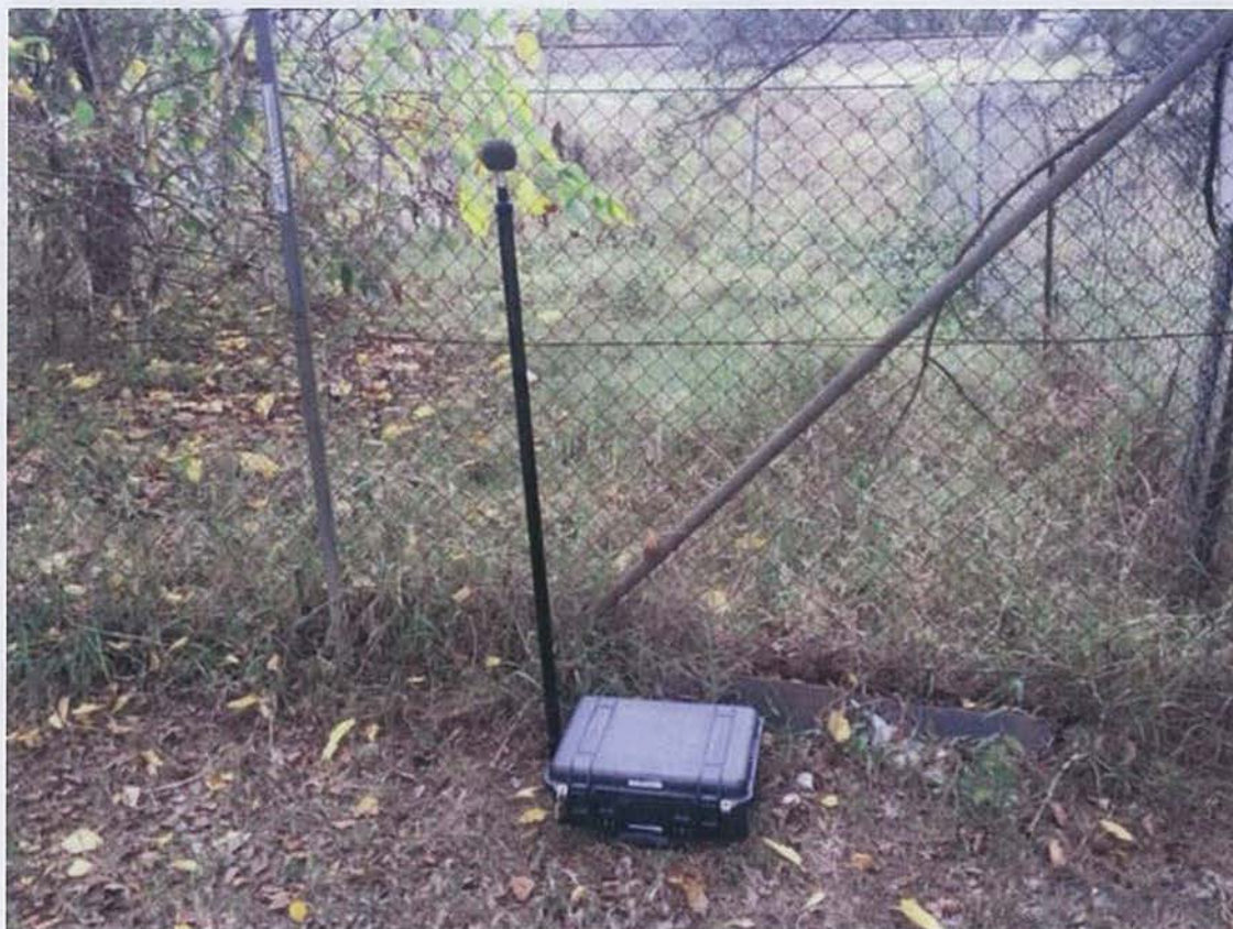
Figure 3: Long Term Noise Survey Logger Setup
